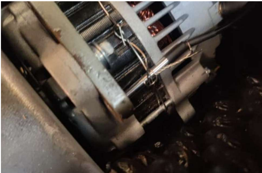
A temperature sensor mounted on the alternator.
