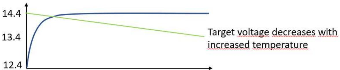
As you can see the target voltage is reached very soon, and if the regulator decreases the target voltage with increased temperature, the target will be reached even earlier (where the lines crosses)
