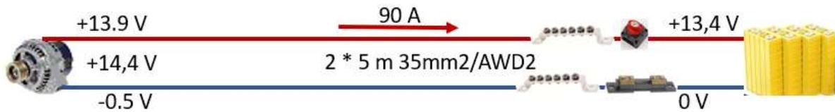
When charging with 90 A there can easily be 0.5 V loss on each cable, which means that the alternators voltage reading is 14.4 V when the voltage at the battery is 13.4 V. This means that the alternator will start decreasing its output almost immediately. For a lead battery this is not so important since it will anyway decrease its hunger for amps very soon as the voltage increases.
