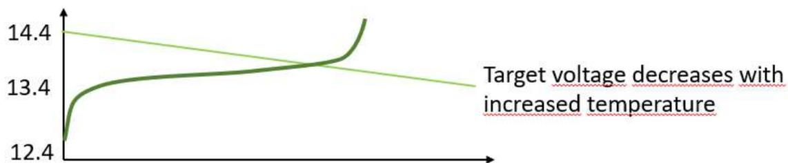
As you can see the alternator will get a lot hotter before it reaches the target 14.4, even if the target is decreased due to increased temperature (where the lines are crossed). It shall also be noted that it is the temperature of the regulator that is measured, and not of the alternator. The alternators internal will be a lot hotter.
